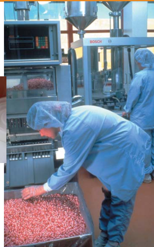
Processing tablets at Astra Zeneca. Production takes place at 20°C, 25% RH with the aid of DST-dehumidifiers.
